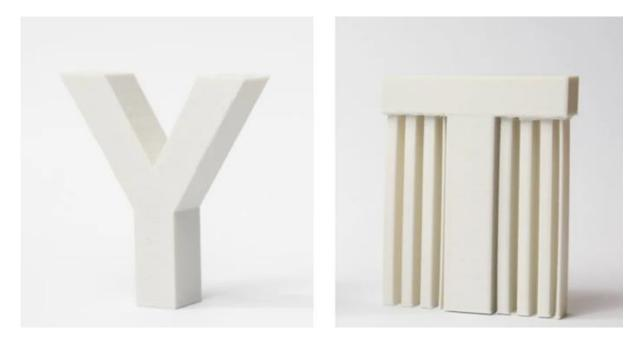
The overhangs in the letter T, on the other hand, have a 90-degree angle with the vertical. So you have to use 3D printing support systems to print the letter T, otherwise as shown below the result would be a mess. When printed with an overhang beyond 45 °, a feature will sag and requires material underneath to keep it up.
