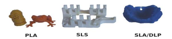
The most fundamental and distinguishing concept behind 3D printing is that it's a method of additive manufacturing. And this really is the key, since 3D printing is a fundamentally different manufacturing process based on innovative technology that creates parts in layers additively. This is radically different from all other conventional manufacturing methods that already exist.
