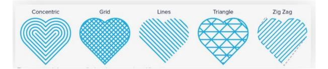
The default support type in Cura is lattice support for grid patterns, which is appropriate because grid patterns serve as a perfect all-purpose support form. But there are actually 7 types of support to choose from under the hood (some of which are pictured above). Pick a support pattern that matches the shape of your model.
