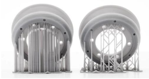
In certain cases, designs are such that they would need to stand on model surfaces if conventional supports were used. Here is where these supports have a distinct benefit. A tree support's "trunk" doesn't enter the model and since the branches come out of the main structure they're only positioned where they're required. In other words, due to the use of supports, the model itself has no artifacts left behind. In the case of organic types like humans and animals, this is especially useful.
