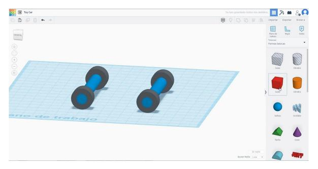
3. Choose the cube shape and size it to 80x50x20 mm and move it to the height of 15 mm. Then align in the center of the set.
