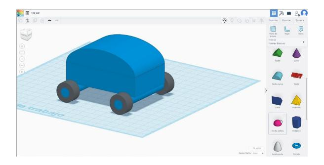
5. Select the shape half sphere, size it to 15x15x7.5 mm and turn it 90 degrees. Move it 17 mm in height and align with the right part of the cube. Then duplicate the half sphere to make the second light.
