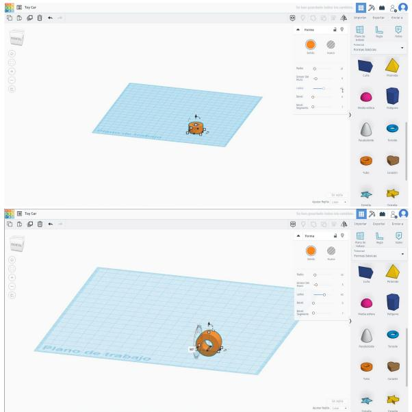
2. Choose the cylinder shape, size it to 10x10x80 mm, turn it 90 degrees and align it with in the center of the tube. Then copy the tube and move it to the opposite side to make the second wheel and copy all the set 60 mm to the left side.
