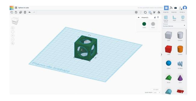
4. Choose the sphere shape and size it to 35x35x35 mm and align in the X and Y axis with the cube.
