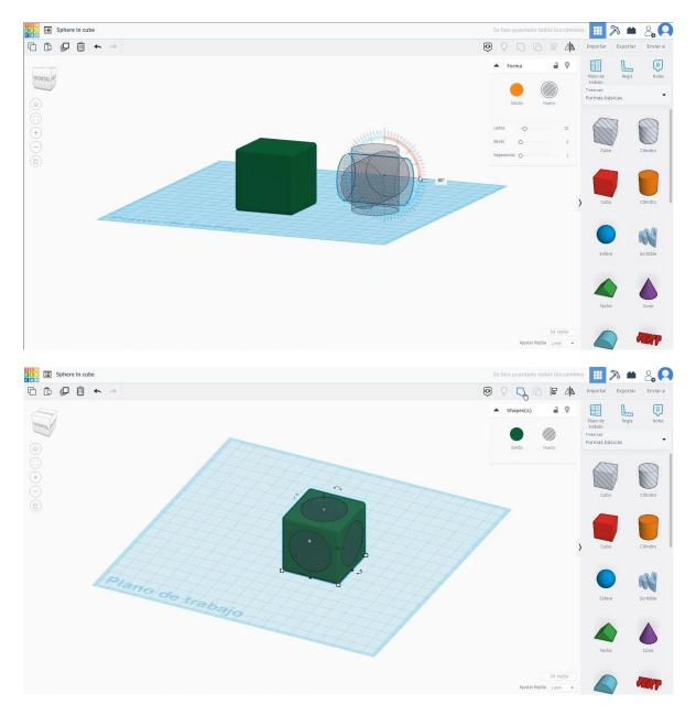
3. Choose the sphere shape and size it to 40x40x40 mm in hole mode and align it with the cube all the axis. Select both objects and press group.
