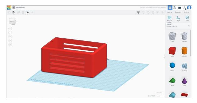
6. Choose the cube shape in hole mode and size it to 140x40x5 mm with radius 1 mm and move it to the height of 10 mm. Then align in the center of the first cube and make sure it appears in both sides.
