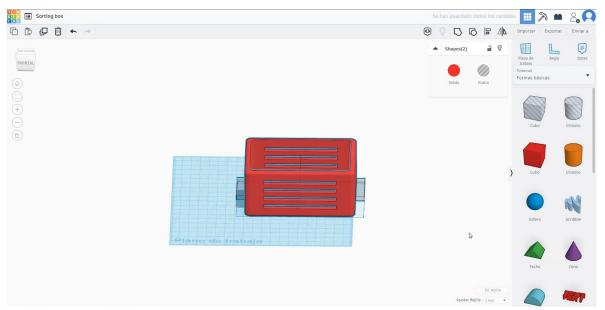
7. Select the cube in hole mode, press duplicate and move it 20 mm in height. Then press two times duplicate to make it automatically. After that, select all the objects and press group.
