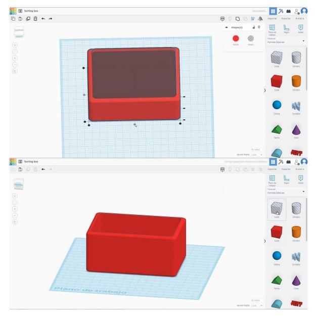
4. Choose the cube shape in hole mode and size it to 80x100x5 mm with radius 1 mm and move it to the height of 10 mm. Then align in the center of the first cube and make sure it appears in both sides.
