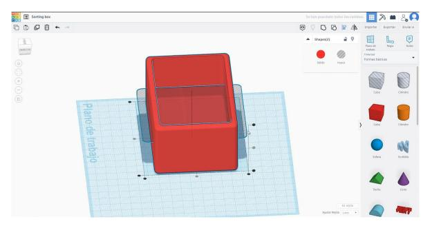
5. Select the cube in hole mode, press duplicate and move it 20 mm in height. Then press two times duplicate to make it automatically. After that, select all the objects and press group.
