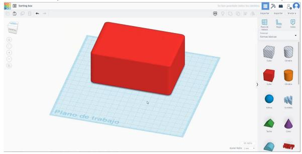
2. Choose the cube shape in hole mode and size it to 110x70x60 mm with radius 1 mm and move it to the height of 5 mm
