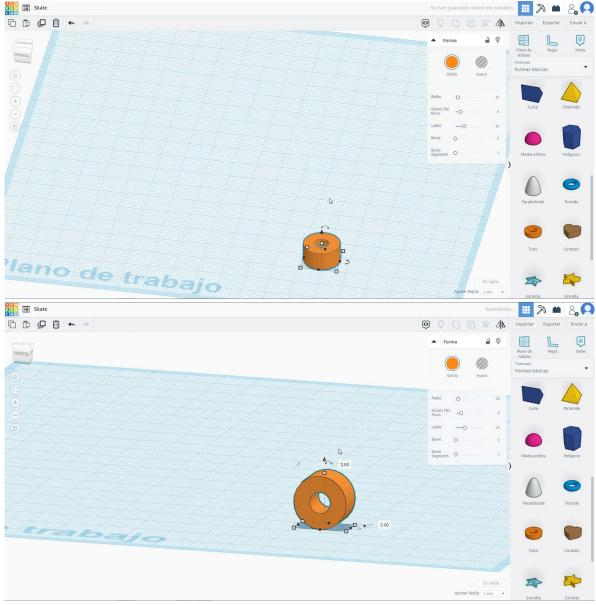
2. Choose the cylinder shape, size it to 6x6x50 mm, turn it 90 degrees and align it with in the center of the tube. Then copy the tube and move it to the opposite side to make the second wheel and copy all the set 50 mm to the left side.
