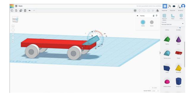
5. Select the round roof shape and press duplicate + mirror and move it to the left edge of the cube. Select the cube and the two round roof and press group.
