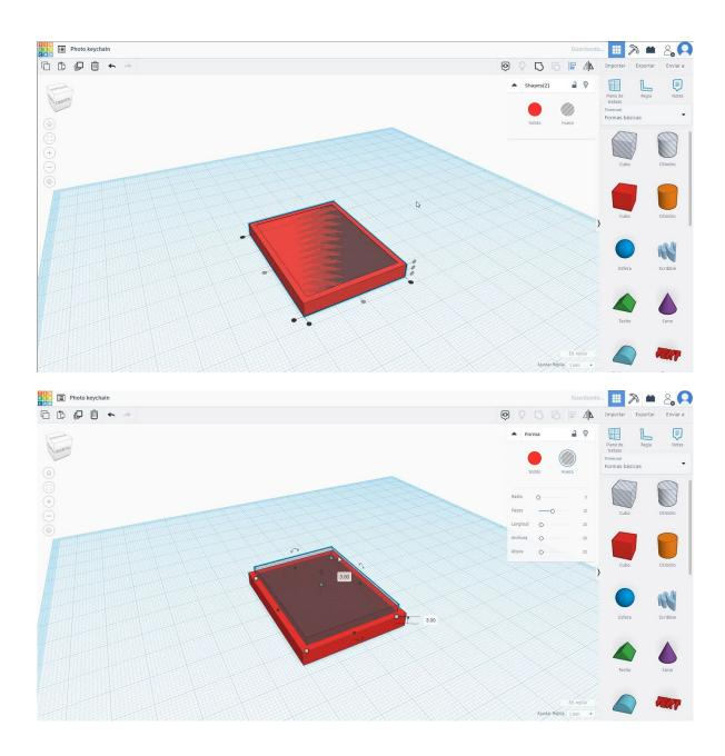
3. Duplicate the second cube in hole mode and size it to 35x50x0.5 mm, align it only in X axis. Make sure the 2 cubes in hole mode are in 3 mm height. Select the 3 objects and press group.
