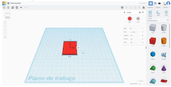
2. Duplicate the cube shape in hole mode and size it to 33x43x5 mm, align it with the first cube and move it to the height of 3 mm
