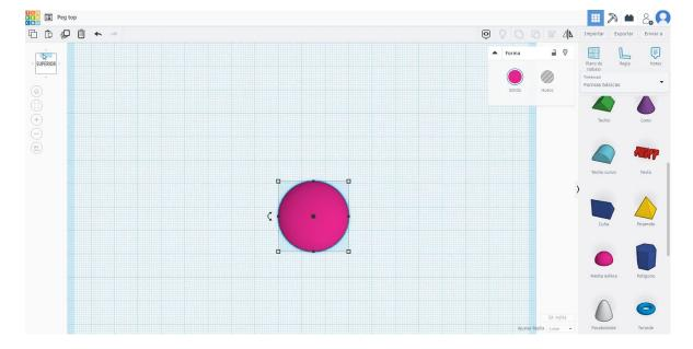
3. Select the cylinder and size it to 5x5x10 mm and move it to the height of 44 mm and centrate it with the half sphere.
