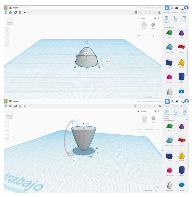
2. Select the half sphere and size it to 30x30x15 mm and move it to the height of 30 mm. Then centrate with the parabolid.
