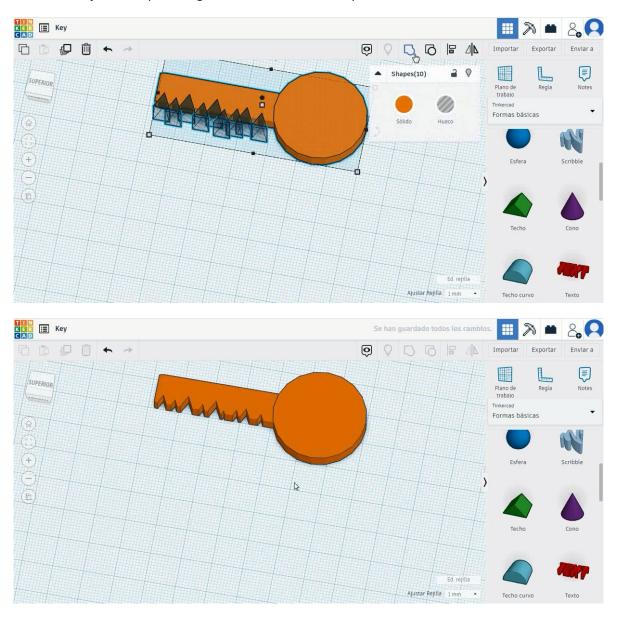
6. Choose the cube shape in hole mode and size it to 8x15x5 mm with radius 1 mm and move it to the height of -3 mm. Then align in the Y axis and move it to the cylindrical part of the key. Select both objects and press group.
