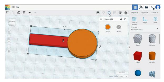
4. Choose the roof shape in hole mode size it to 5x5x20 mm and move it 90 degrees. Then move it to the left part of the key and duplicate it moving it up and down to create the different clefts.
