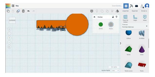
5. Select all the objects and press align to remove the roof shape.
