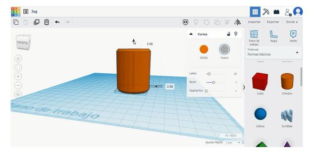
3. Select a new cylinder and move it to the height of 50 mm. Align in the center of the first cylinder.
