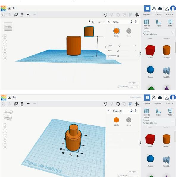
4. Duplicate the second cylinder, select hole mode and size it to 18x18x25 mm. Then move it to the height of 47 mm and align in the center.
