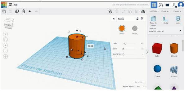
2. Duplicate the cylinder and select hole mode. Size it to 38x38x46 mm, align in the center of the first cylinder and move to the height of
