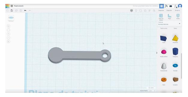
4. Choose the polygon shape and size it to 17x14.32x5 mm in hole mode, turn it 90 degrees and align it with the wrench in Y axis. Move it 14 mm from left first touch each other.
