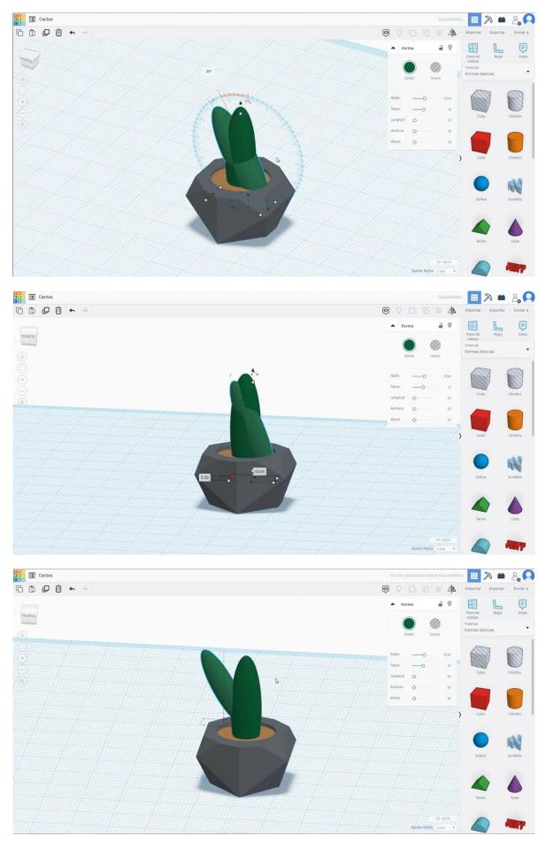
Duplicate the second cube turning it 22.5 degrees, size it to 8x4x20 mm and move it to the height of 13 mm. Move to the opposite side and align with the first cube.
