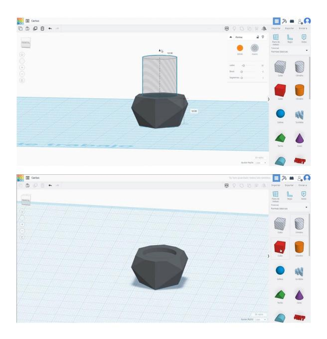
4. Choose cylinder shape and size it to 16x16x1 mm and move it to the height of 12 mm. Then align in the center of the cube.
