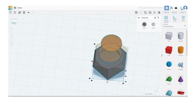
5. Select the shape cube, size it to 8x8x30 mm with 10 mm radius. Move it to the height of 5 mm in height and align in the center.
